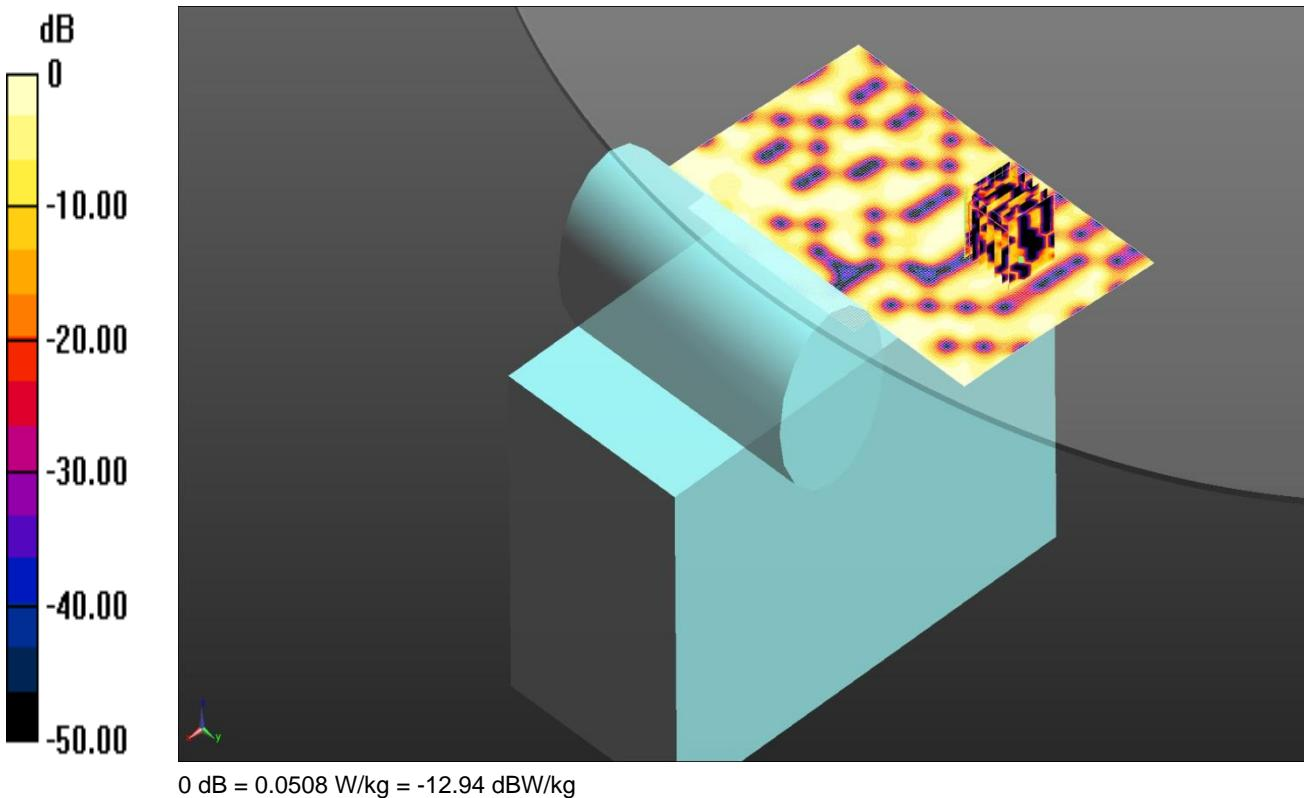
Communication System: UID 0, WLAN 802.11 (0); Frequency: 5280 MHz; Duty Cycle: 1:1
