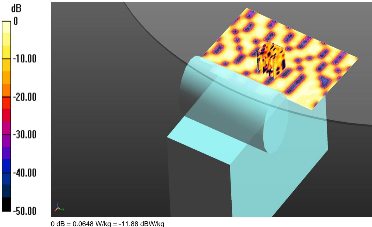
Communication System: UID 0, WLAN 802.11 (0); Frequency: 5320 MHz; Duty Cycle: 1:1
