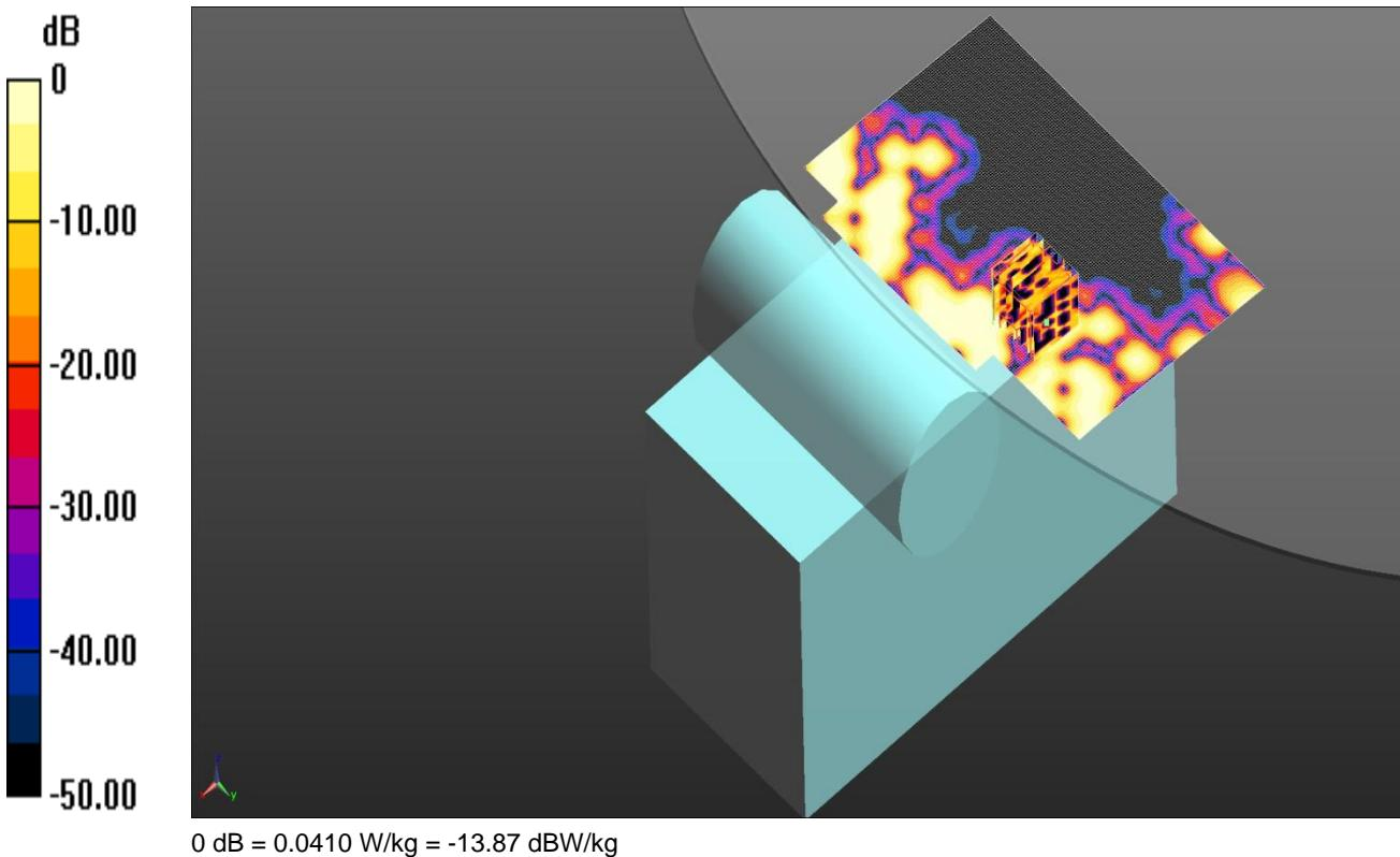
Communication System: UID 0, WLAN 802.11 (0); Frequency: 5260 MHz; Duty Cycle: 1:1
