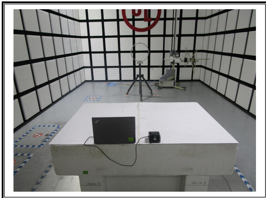
RADIATED RF MEASUREMENT SETUP (Below 30MHz)
