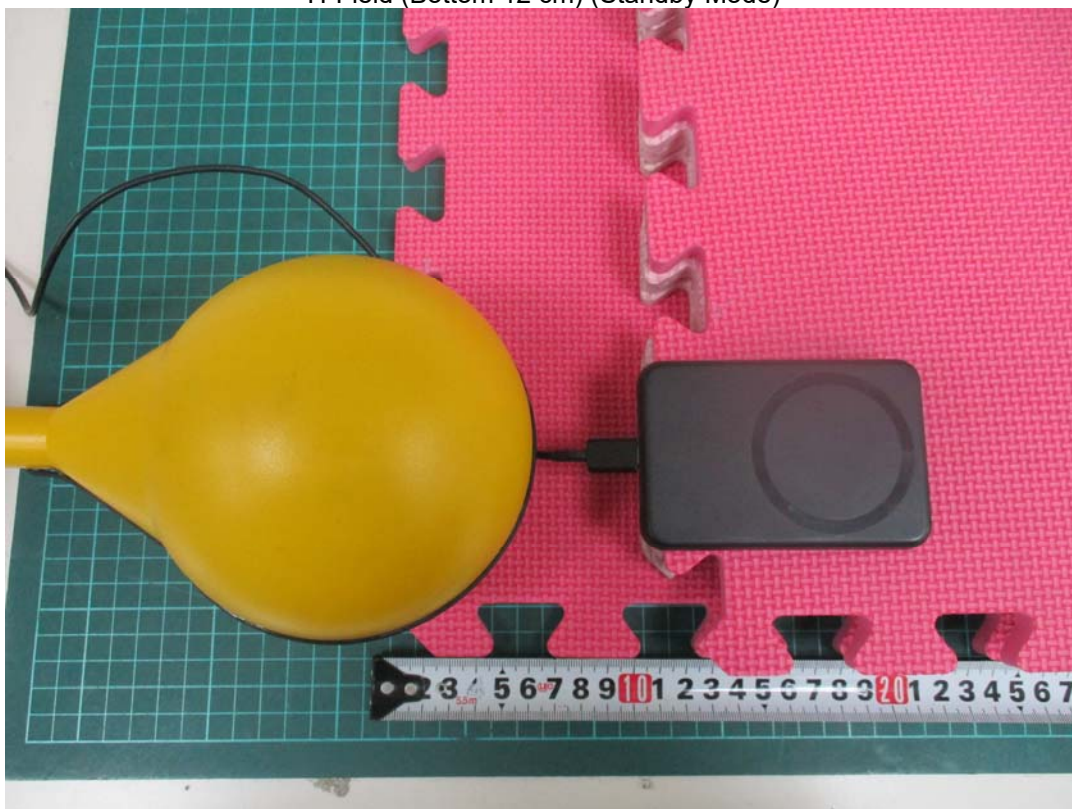
H-Field (Bottom 12 cm) (Standby Mode)
