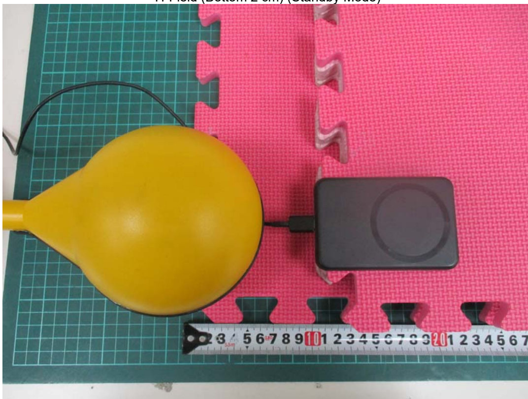
H-Field (Bottom 2 cm) (Standby Mode)
