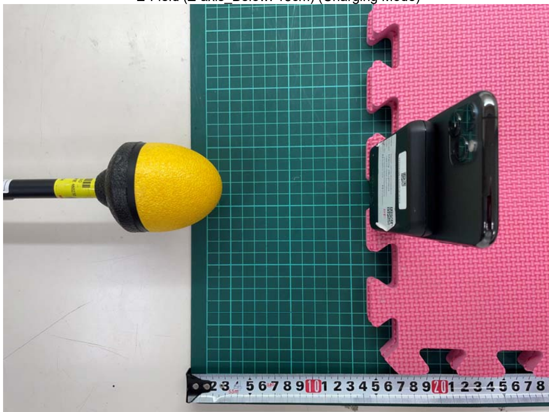
E-Field (Z-axis Below: 15cm) (Charging Mode)
