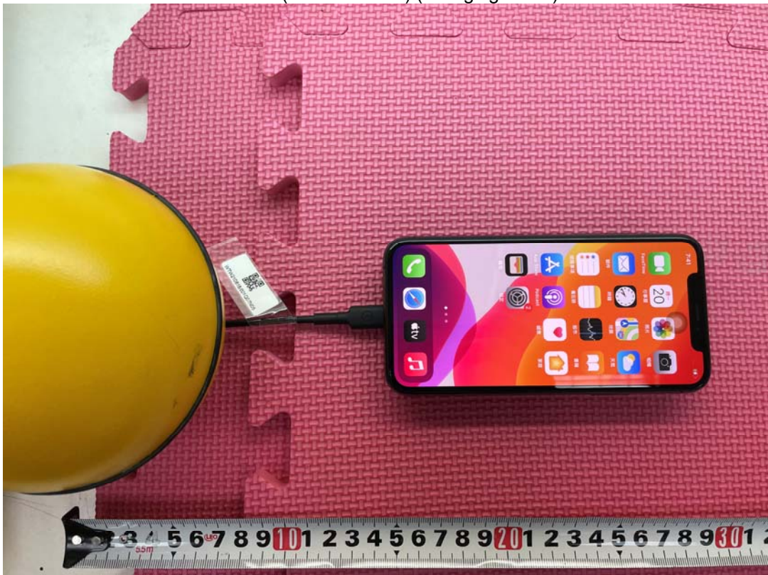
H-Field (Bottom: 15cm) (Charging Mode)
