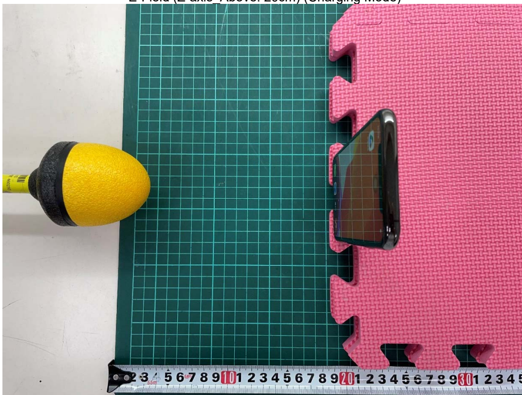
E-Field (Z-axis_Above: 20cm) (Charging Mode)
