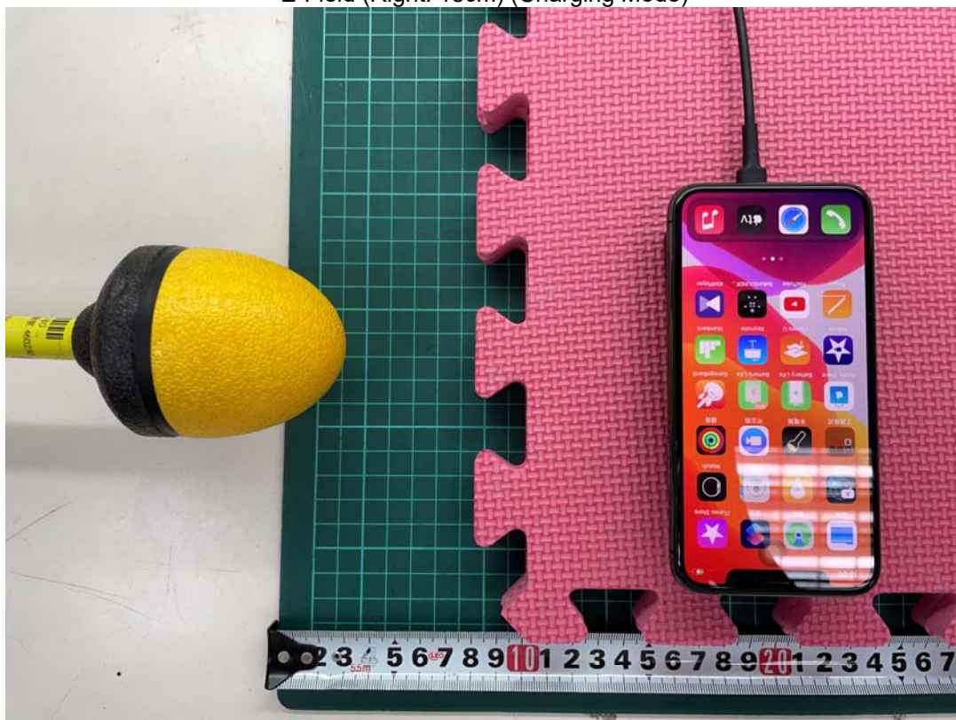
E-Field (Right: 15cm) (Charging Mode)
