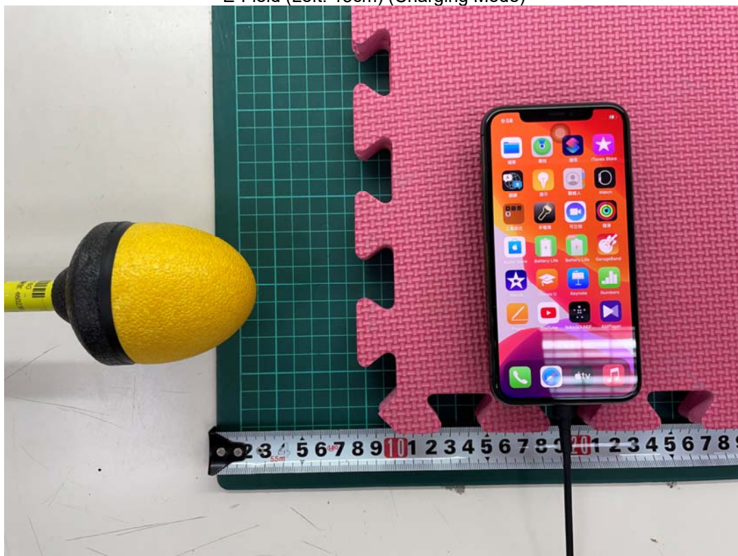
E-Field (Right: 15cm) (Charging Mode)
