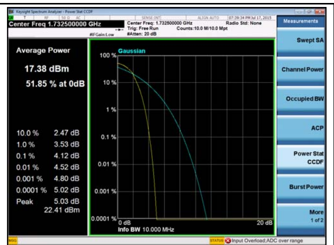
LTE band 4 - Middle CH 16QAM-10
