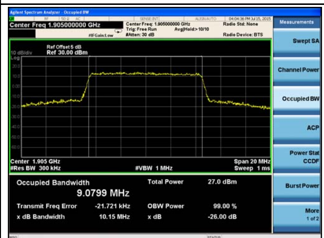
LTE band 2 - Middle CH 16QAM-10
