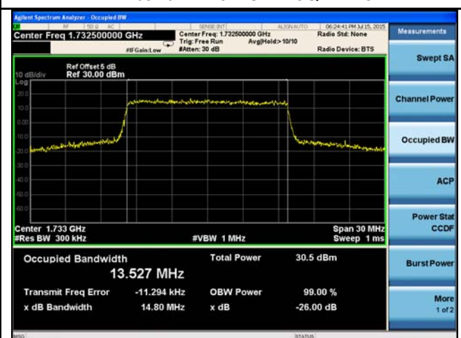
LTE band 4 - Middle CH 16QAM-15
