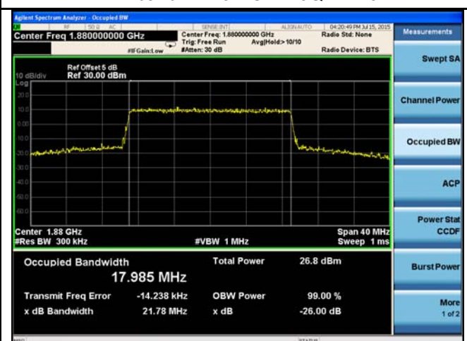
LTE band 2 - Low CH 16QAM-20
