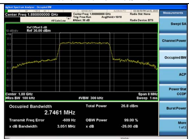
LTE band 2 - Middle CH 16QAM-3
