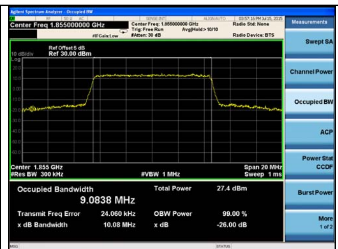
LTE band 2 - Low CH 16QAM-10
