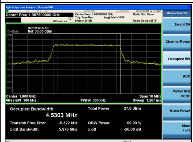
LTE band 2 - Middle CH 16QAM-5
