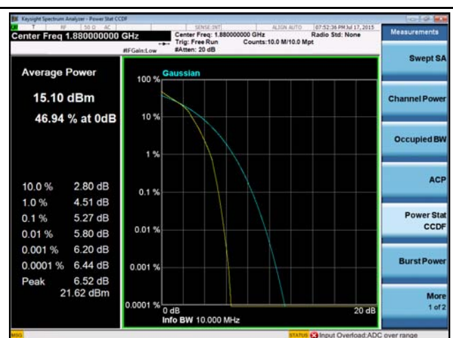
LTE band 2 - Middle CH 16QAM-10
