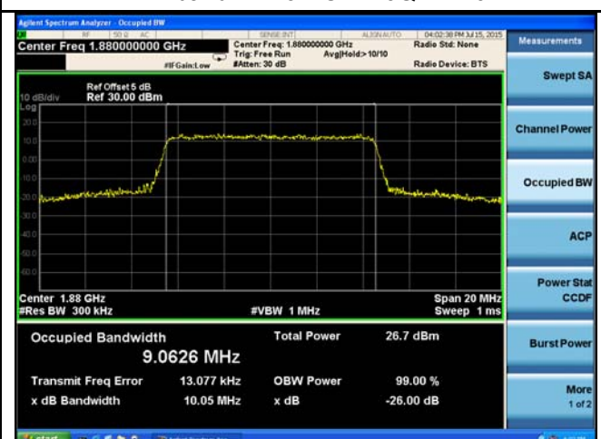
LTE band 2 - Low CH 16QAM-10
