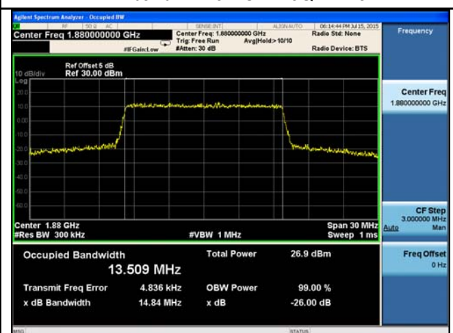
LTE band 2 - Middle CH 16QAM-15
