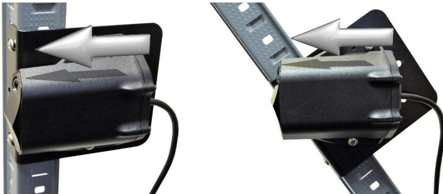
Remember: *A vertical installation is only recommended in countries where horizontally polarized radar guns are in use (e.g. Australia)*
