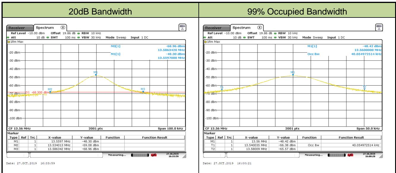
Note: Because the measured signal is CW or CW-like adjusting the RBW per ANSI C63.10 would not be practical since measured bandwidth will always follow the RBW and the result will be approximately twice the RBW, so the RBW was set higher than 5% of the measured bandwidth.
