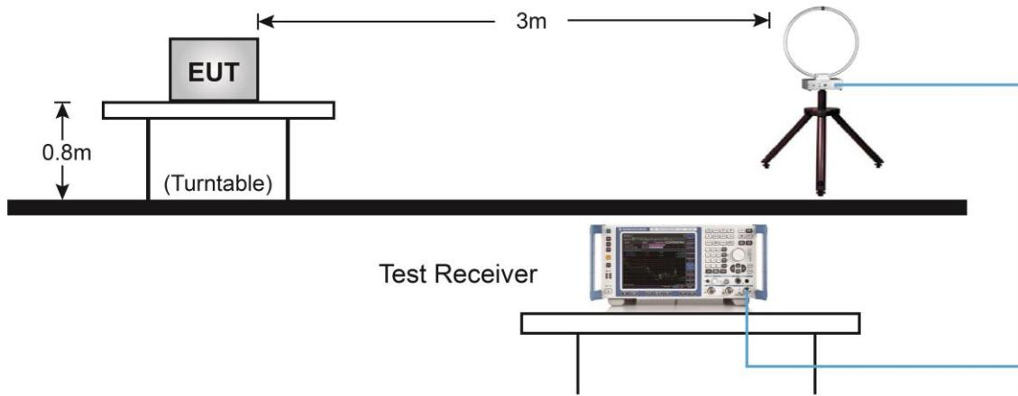
Above 30MHz Test Setup:
