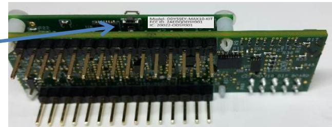
Note: Sticker is attached to board with BLE module on it because it is the only product location with available space and the boards are regularly disassembled by the user as part of product use. ID info also provided in User Manual.
