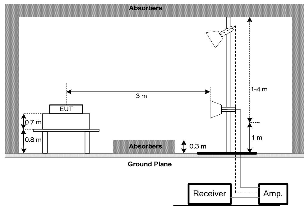
(C) For radiated emissions below 30MHz
