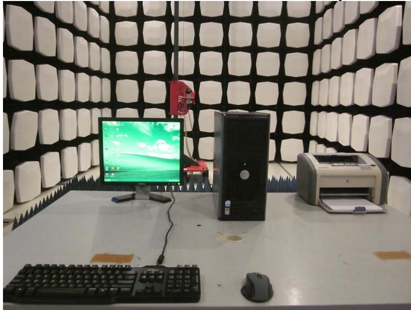
Measurement of Radiated Emission Test Set Up
