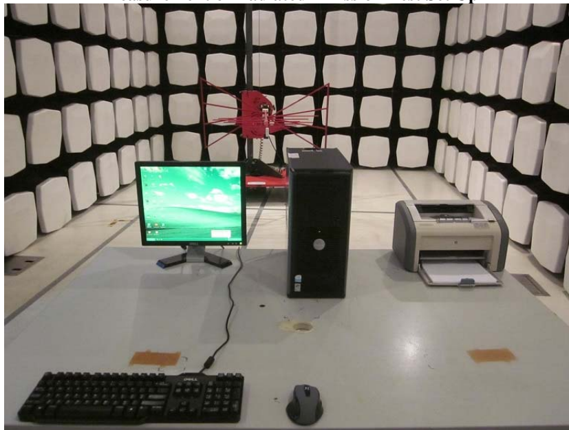
Measurement of Radiated Emission Test Set Up
