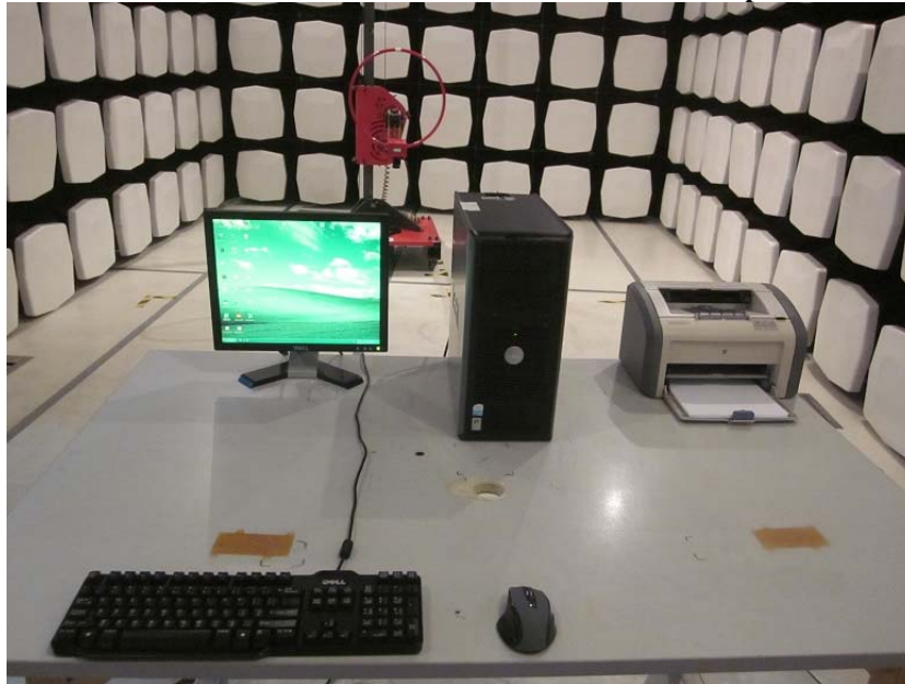
Measurement of Radiated Emission Test Set Up
