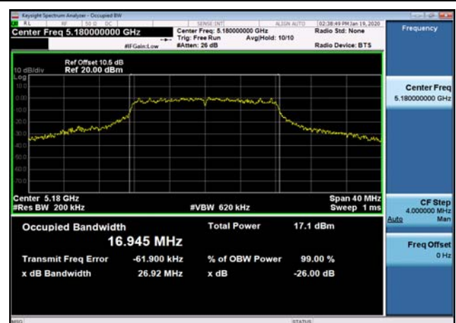
U-NII-1 26dB Bandwidth-802.11a(20MHz) ,5180MHz
