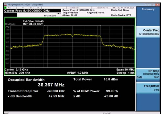
U-NII-1 26dB Bandwidth-802.11a(20MHz) ,5180MHz
