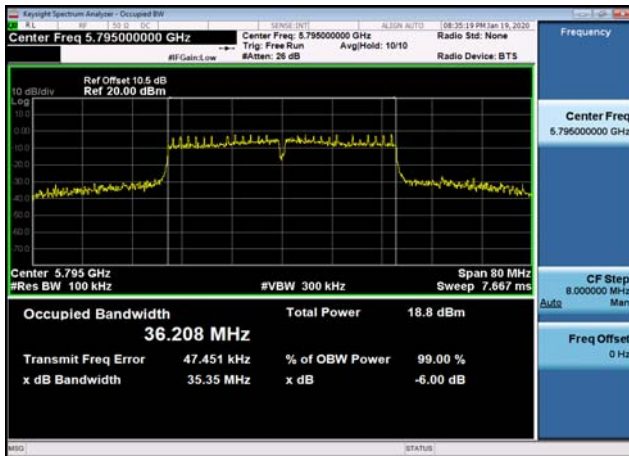
U-NII-3 6dB Bandwidth-802.11a(20MHz) ,5785MHz
