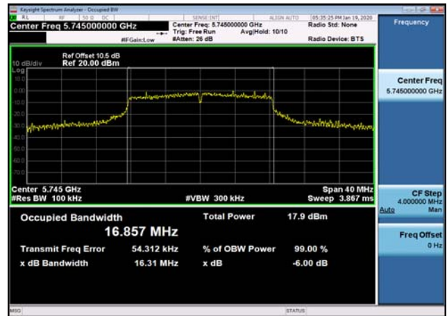
U-NII-3 6dB Bandwidth-802.11a(20MHz) ,5825MHz
