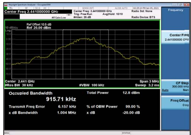
99% Bandwidth: DQPSK,2402MHz,2DH5
