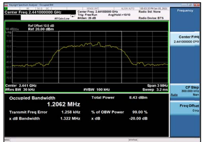
20dB Bandwidth: 8DPSK,2441MHz,3DH5
