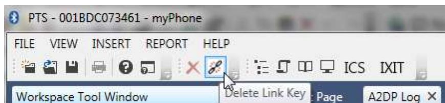
Once the "Delete Link Key" button has been pressed, the devices are no longer bonded.
