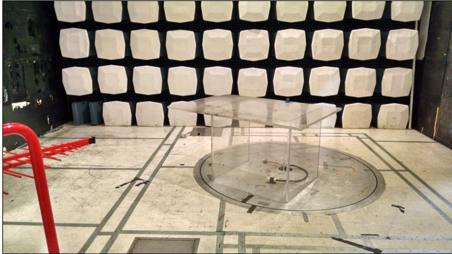
Photograph 1. Radiated Spurious Emissions, 30 MHz – 1 GHz Test Setup
