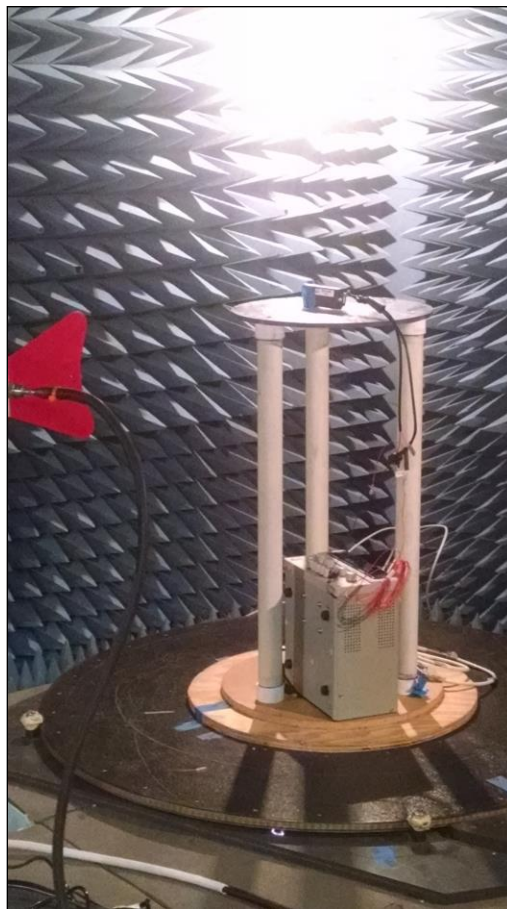
Photograph 2. Radiated Spurious Emissions, 1 GHz – 18 GHz Test Setup
