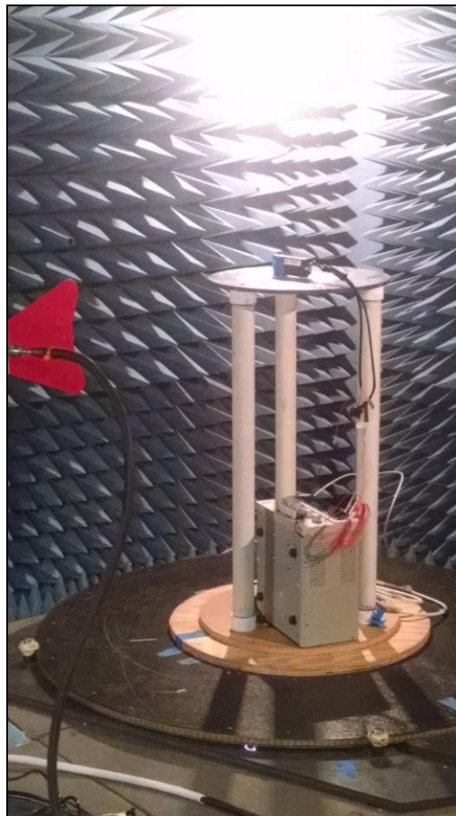
Photograph 3. Radiated Spurious Emissions, 1 GHz – 18 GHz Test Setup
