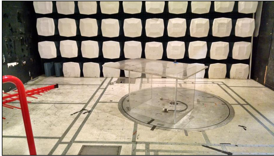
Photograph 2. Radiated Spurious Emissions, 30 MHz – 1 GHz Test Setup
