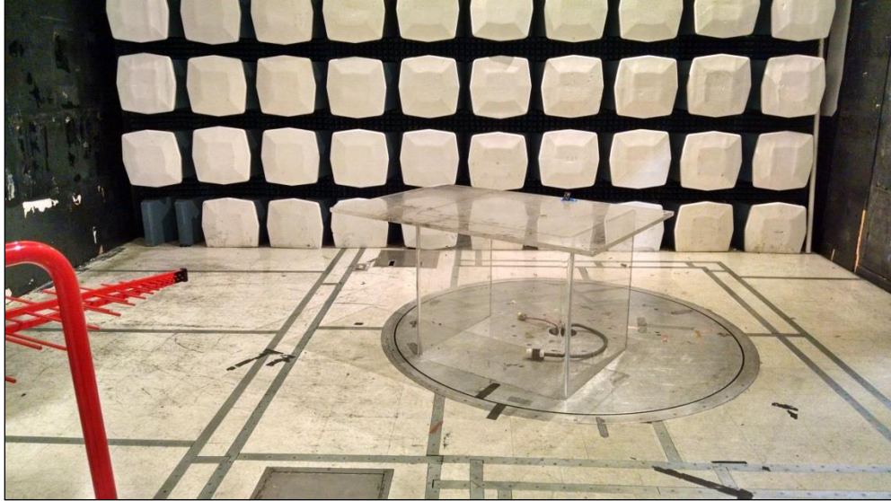
Photograph 1. Radiated Spurious Emissions, 30 MHz – 1 GHz Test Setup
