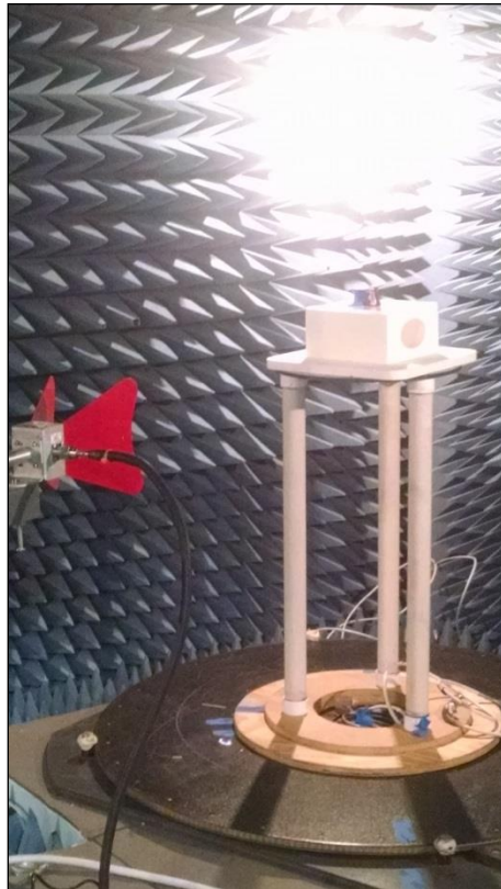
Photograph 2. Radiated Spurious Emissions, 1 GHz – 18 GHz Test Setup
