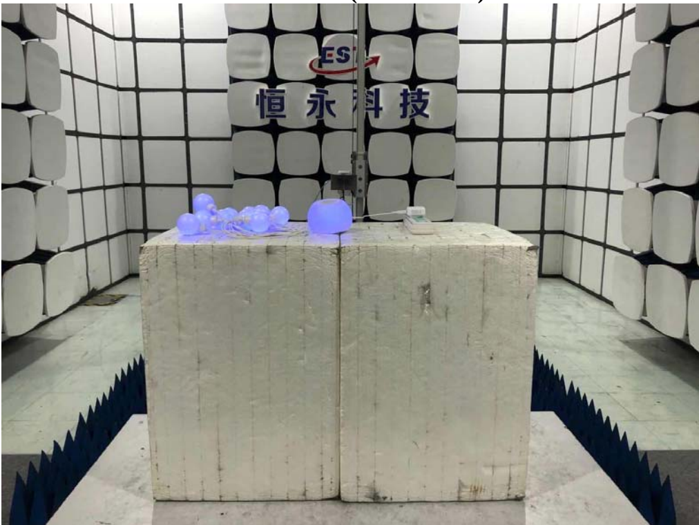
Radiated Test (Above 1GHz)
