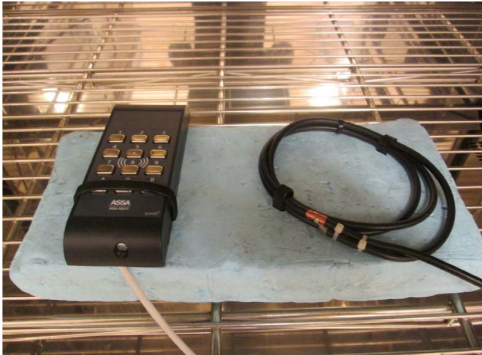
Photo 4.5.1.2 Test setup regarding test with extreme conditions with antenna and test object fixed mounted on a piece of polystyrene inside the climate chamber.
