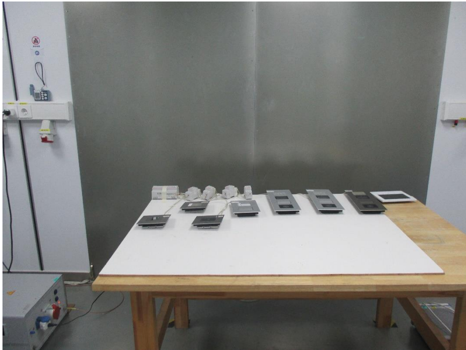
Setup photo of conducted emission (150KHz-30MHz)
