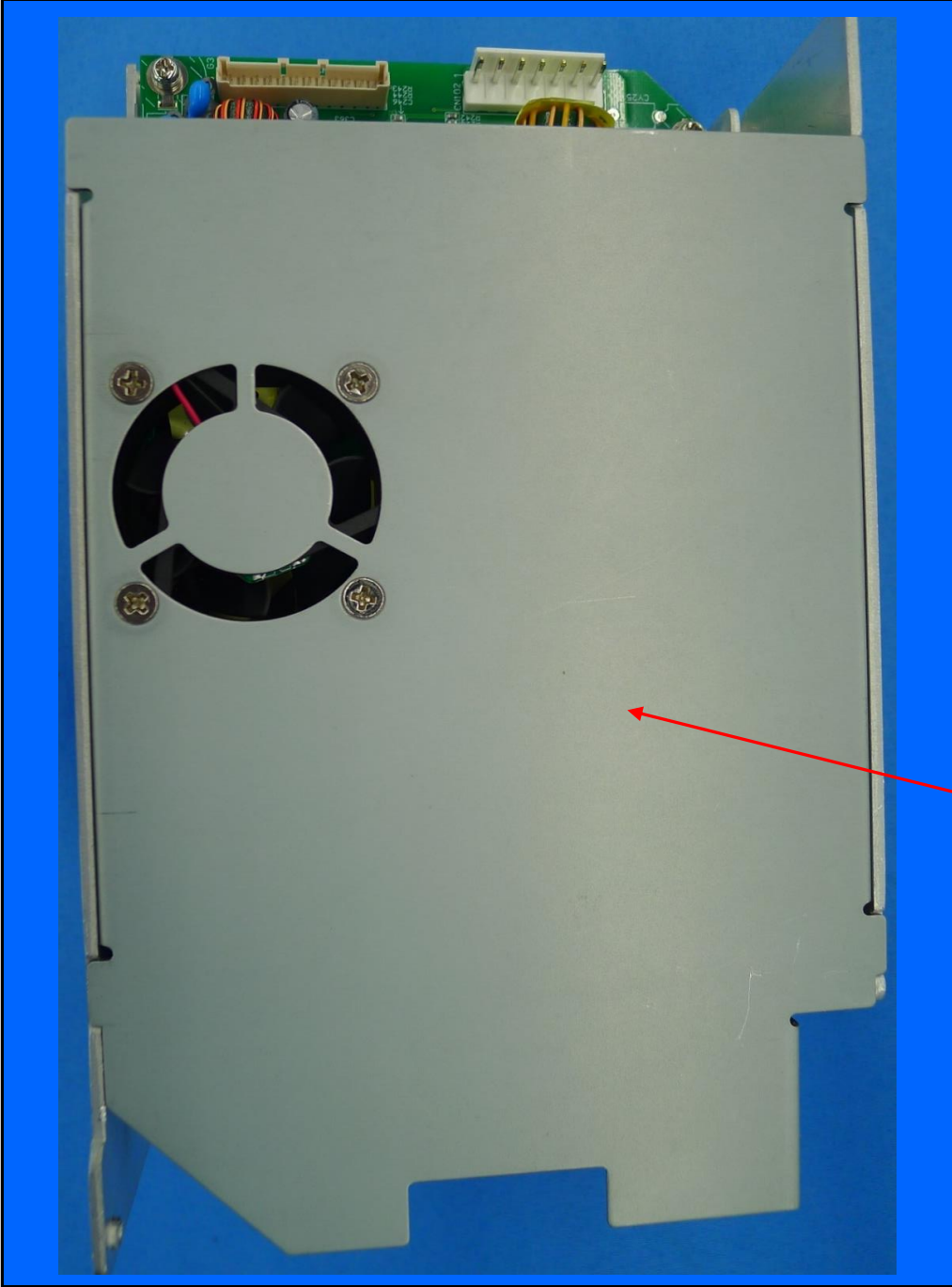
POWER SWITCHING BOARD
