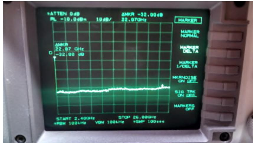
**Spurious Emissions Plot – 1 GHz to 2.4 GHz**
