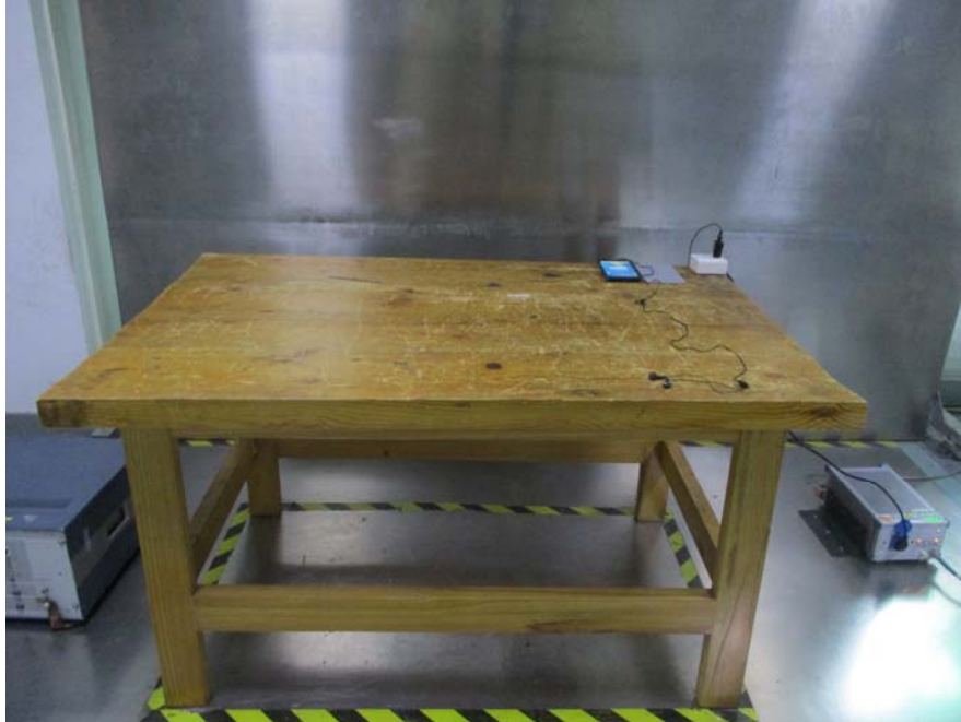
Conducted Emissions – Front View
