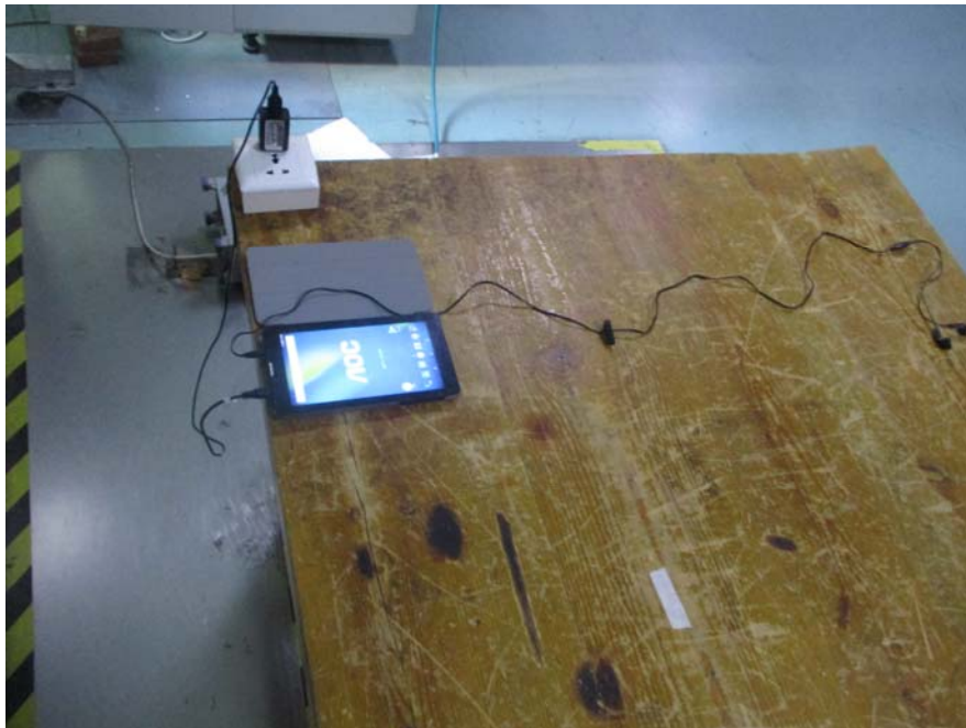
Conducted Emissions – Side View
