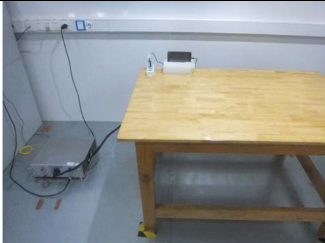
Conducted Emissions Test Setup Front View
