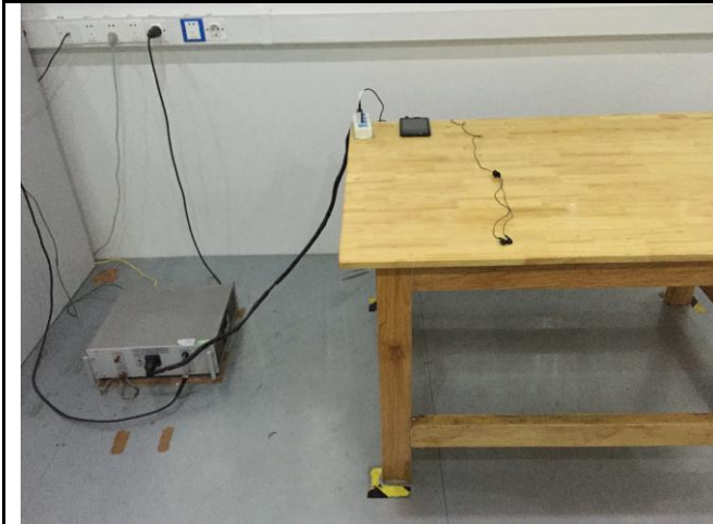
Conducted Emissions Test Setup – Front View
