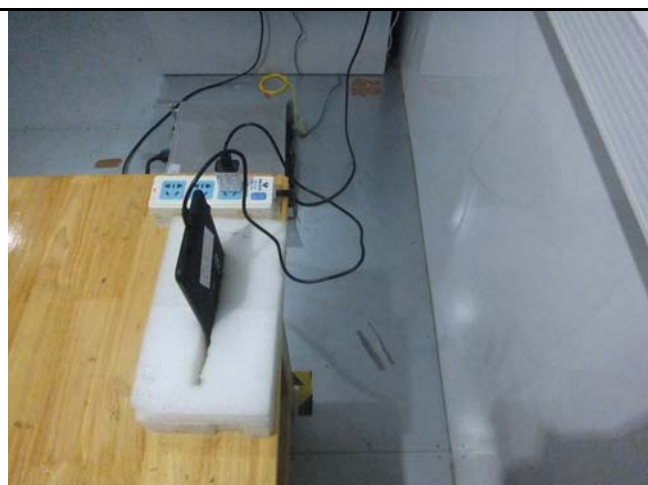
Conducted Emissions Test Setup Side View
