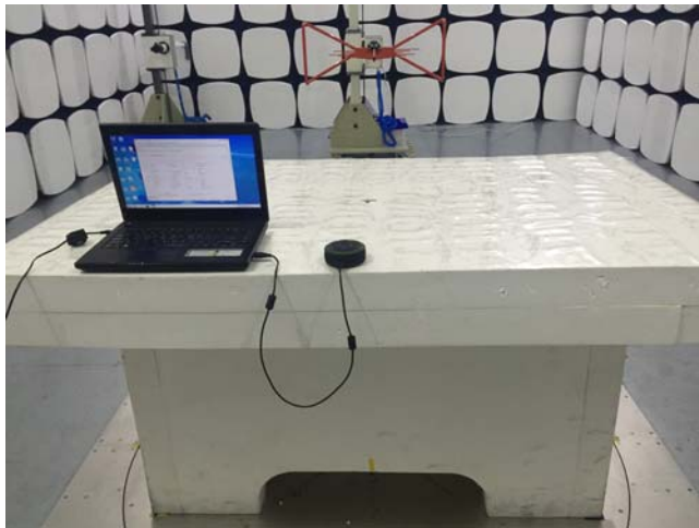
Radiated Spurious Emissions Test Setup Below 1GHz
