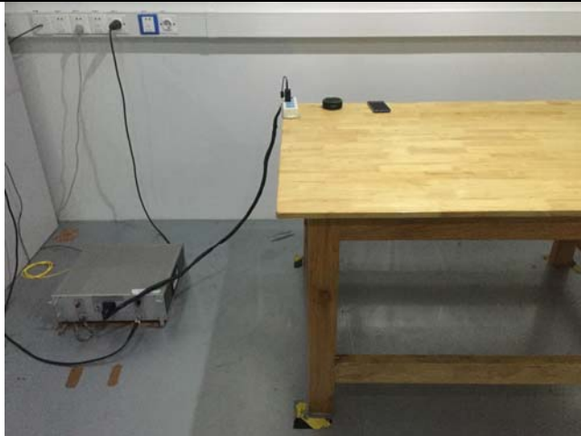
Conducted Emissions Test Setup Front View
