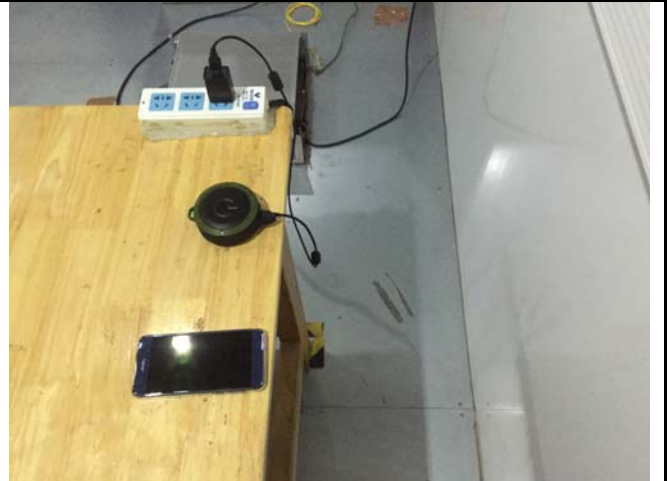
Conducted Emissions Test Setup Side View
