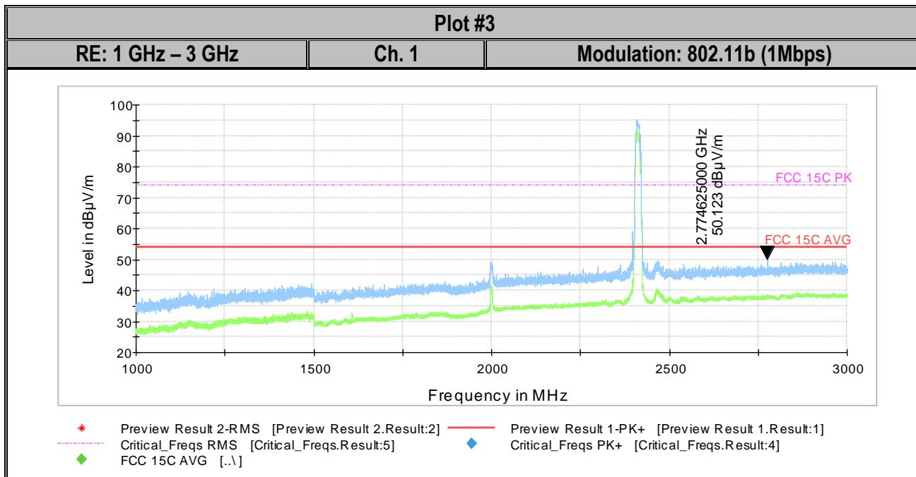
Note: The emission above the limit is the Tx Ch.1.
