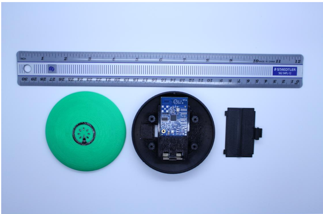
Enclosure top, top and battery door removed
