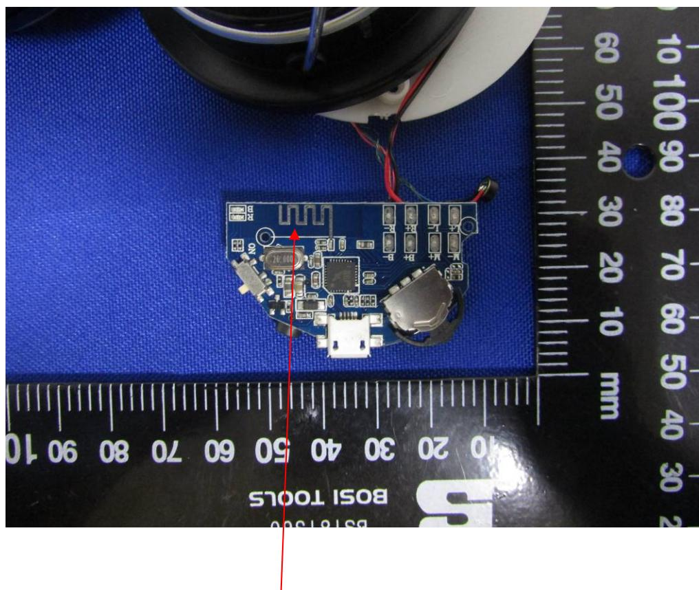
This is a Integral Antenna, antenna gain is 0dBi.
