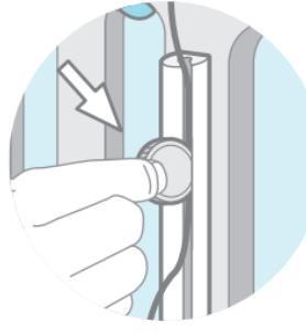
3. Use **COIN** to push **USB CABLE** deep into the gap of **CABLE GUIDE**
