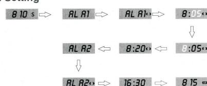
a. The time will be displayed once power is switched on - simply press the **ALARM** button to switch between Alarm 1 and Alarm 2 settings.
