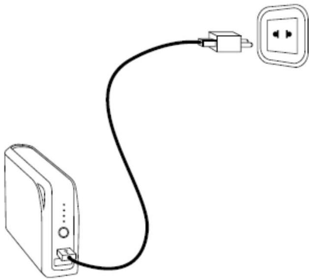
Please connect the USB cable to the Airbank with Micro USB plug and to the Charger with USB plug. When the power indicator LEDs lighten on and the enviroment indicator LEDs rotate, then you can hear a buzzer. After that you will have finished the activation.
