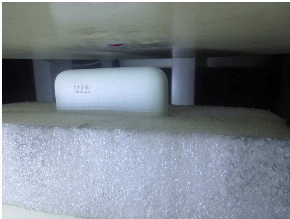
10mm Hotspot mode Bottom Edge Setup Photo
