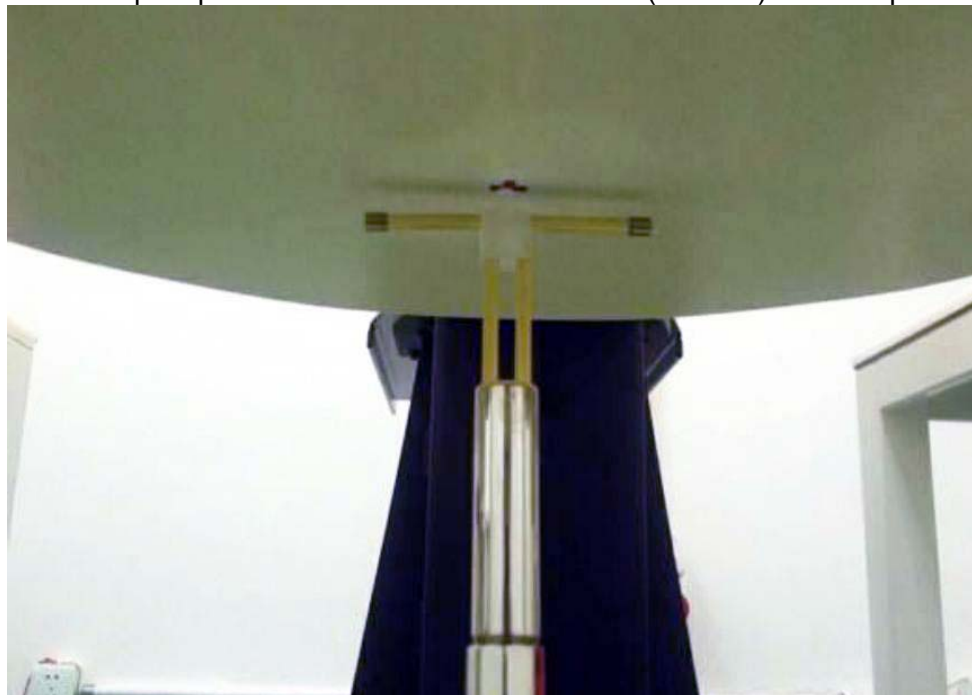
Photo of Dipole Setup
