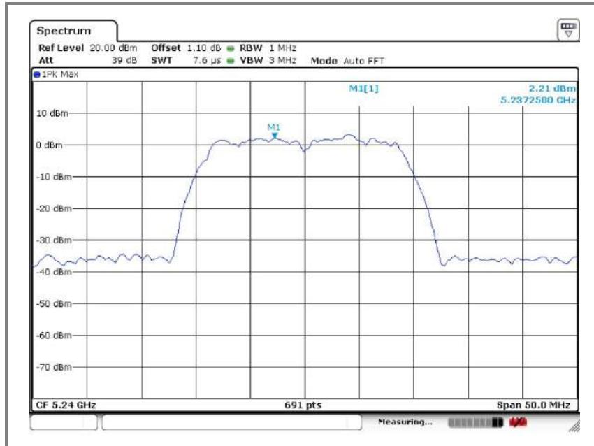
**Operation mode: U-NII-1(n\_HT20)****A. Low channel(5180 MHz)**
