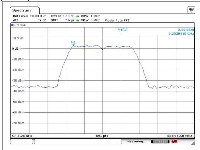
**B. Middle channel(5300 MHz)**
