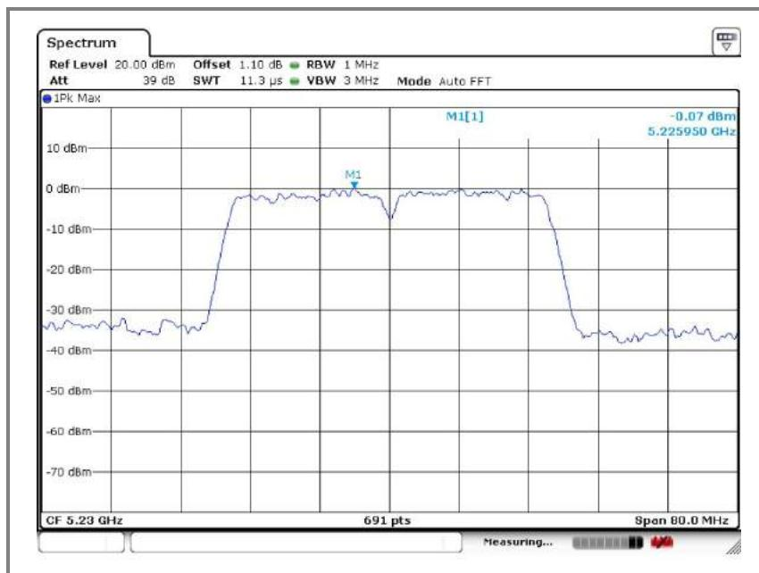
**Operation mode: U-NII-1(VHT80)****A. Low channel(5210 MHz)**
