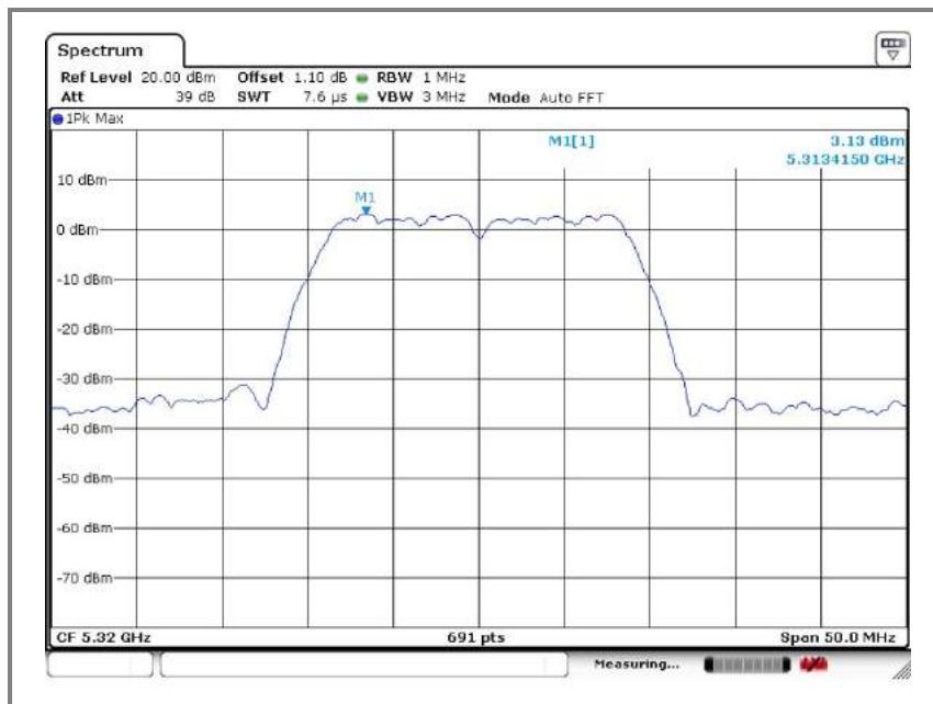
**Operation mode: U-NII-2A(n\_HT20)****A. Low channel(5260 MHz)**
