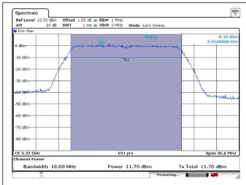
**Operation mode: U-NII-2A(n\_HT20)****A. Low channel(5260 MHz)**
