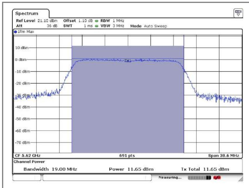
**Operation mode: U-NII-2C(n\_HT40)****A. Low channel(5510 MHz)**
