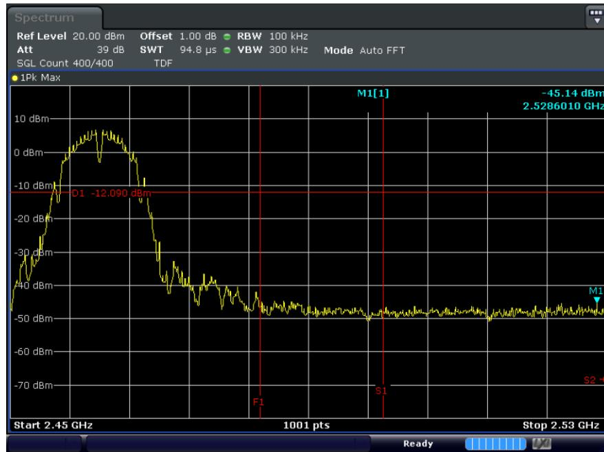
**C.2. Highest Ch. (2 462 MHz)\_Spurious emissions**
