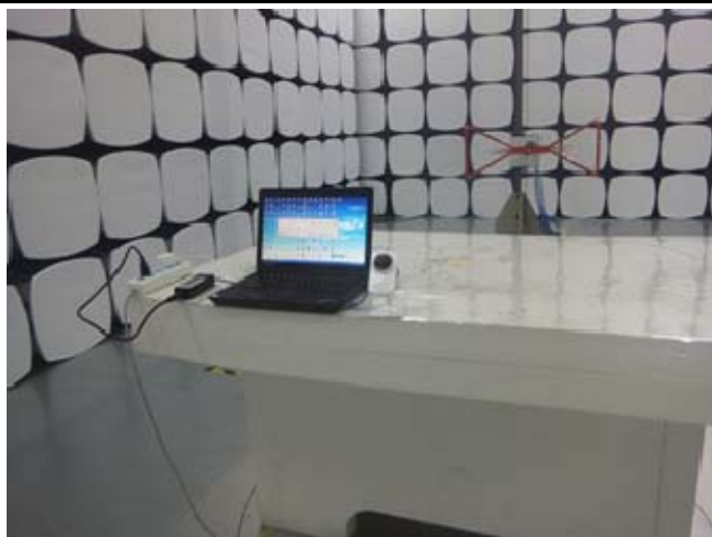
Radiated Spurious Emissions Test Setup Below 1GHz Adapter 2
