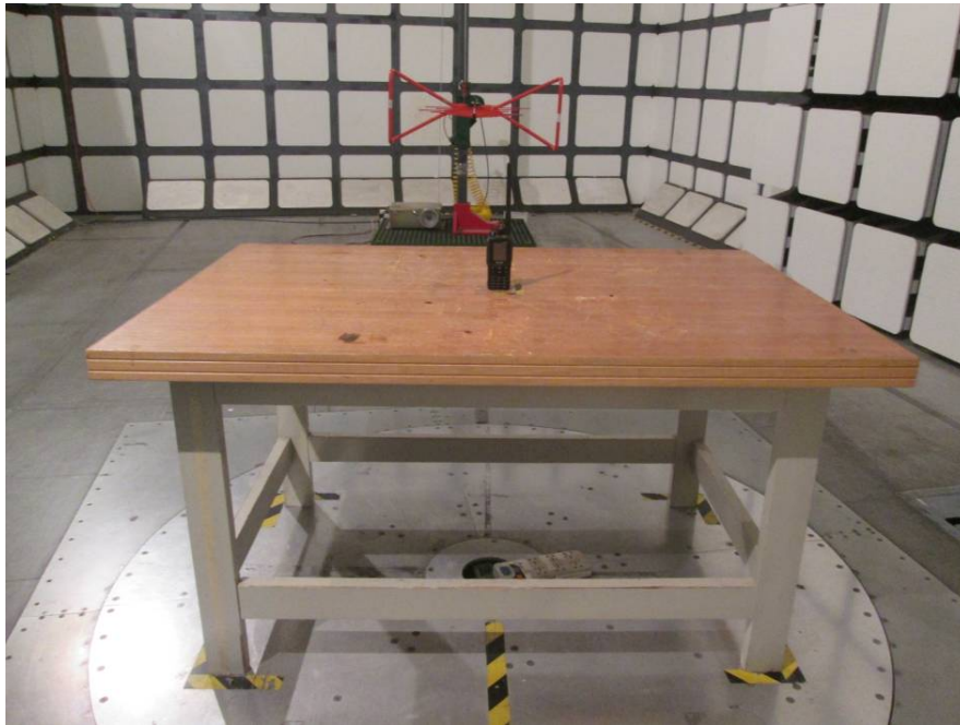
Radiated Emissions Tested View (Below 1GHz)
