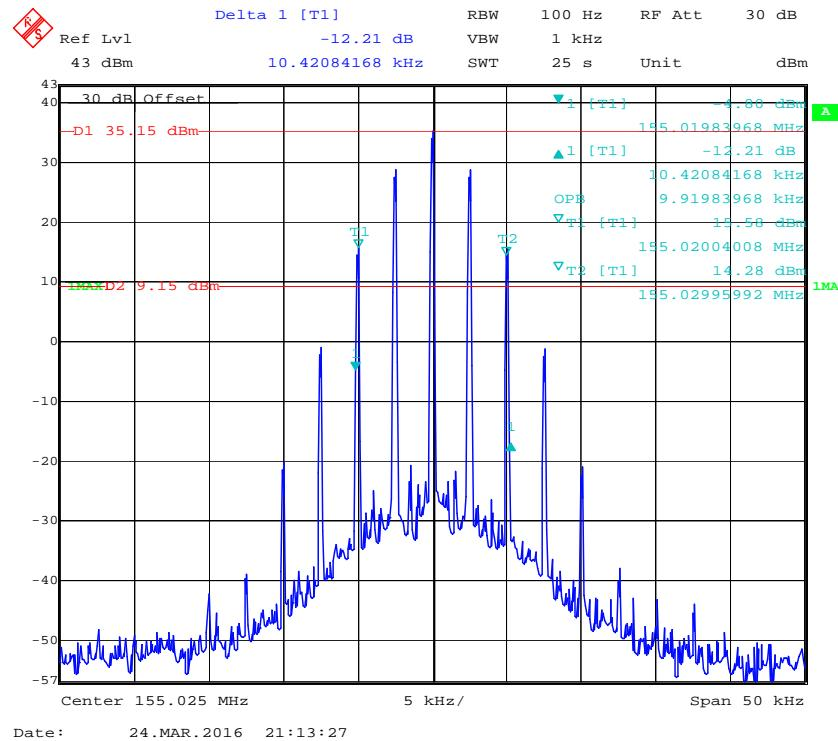
**99% Occupied Bandwidth & 26 dB Emissions Bandwidth 12.5 kHz, 155.025 MHz (Low Power)**
