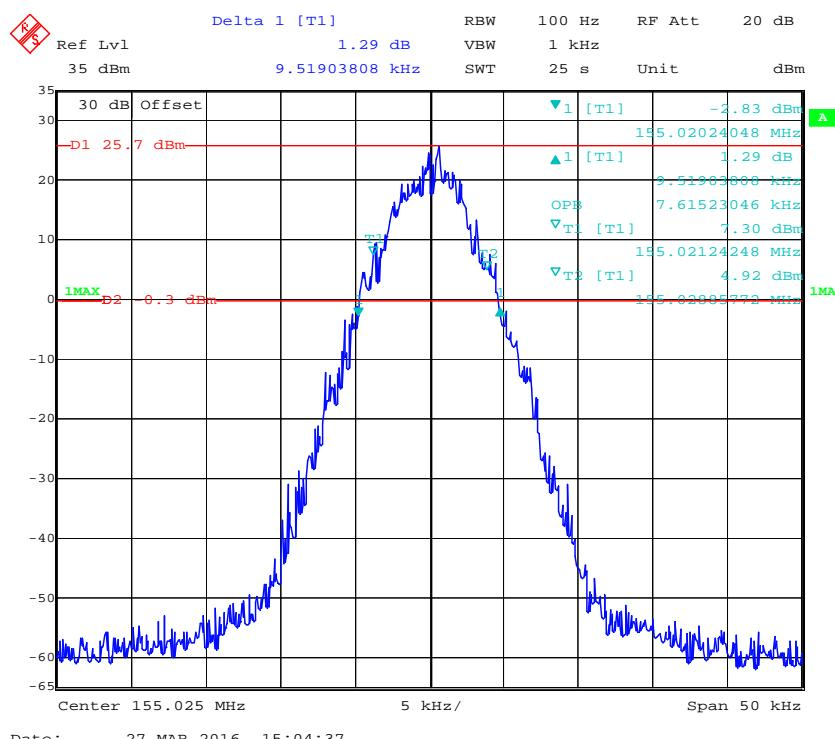
**Emission Mask D with High Power 12.5 kHz, 155.025 MHz**
