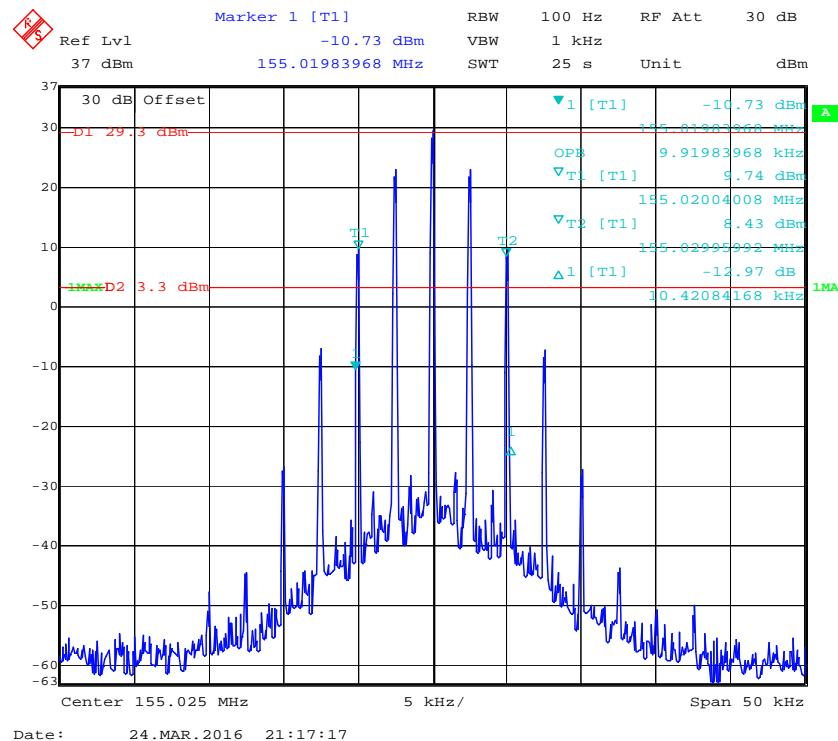
**Emission Mask D with High Power 12.5 kHz, 155.025 MHz**
