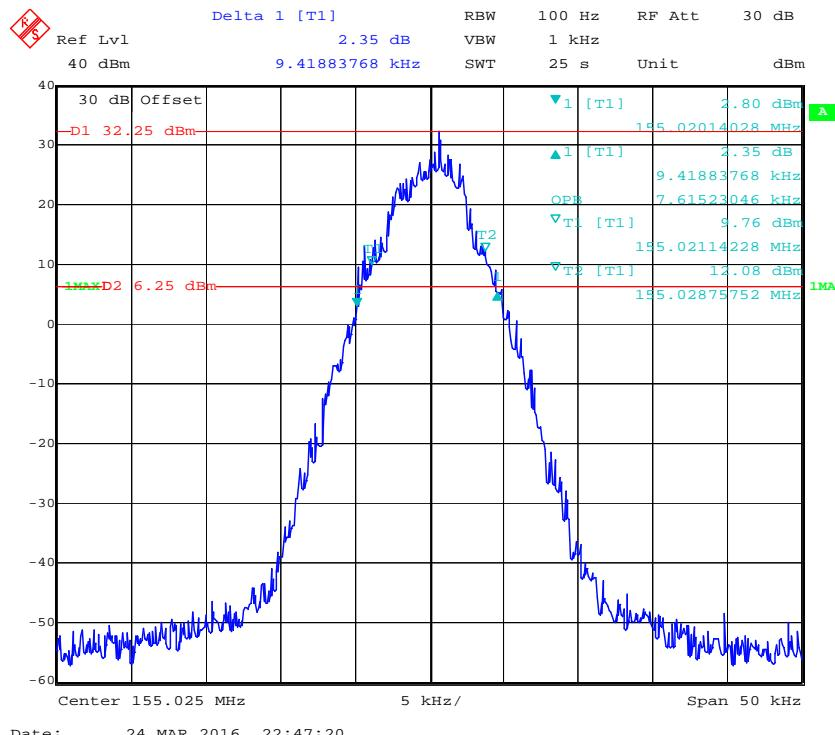
**99% Occupied Bandwidth & 26 dB Emissions Bandwidth 12.5 kHz, 155.025 MHz (Low Power)**
