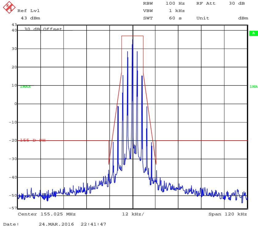
**Emission Mask D with Low Power 12.5 kHz, 155.025 MHz**
