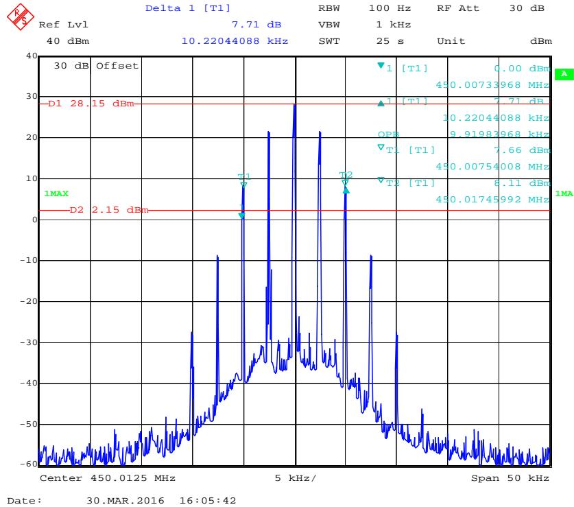
**Emission Mask D with High Power 12.5 kHz, 450.0125 MHz**
