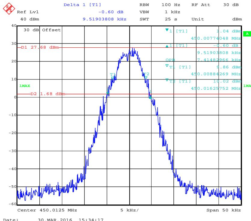
**99% Occupied Bandwidth & 26 dB Emissions Bandwidth 12.5 kHz, 450.0125 MHz (Low Power)**
