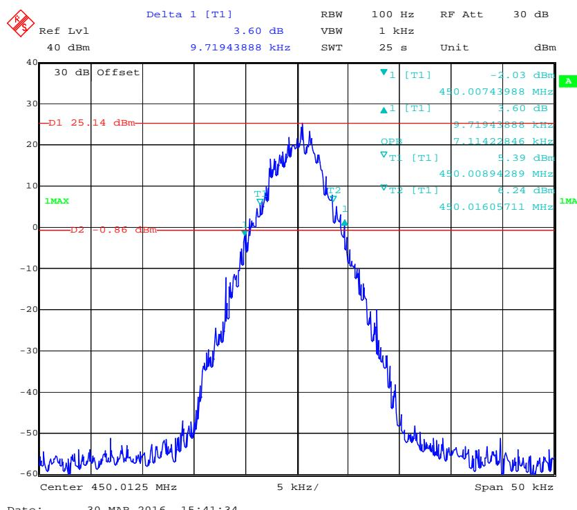
**Emission Mask D with High Power 12.5 kHz, 450.0125 MHz**
