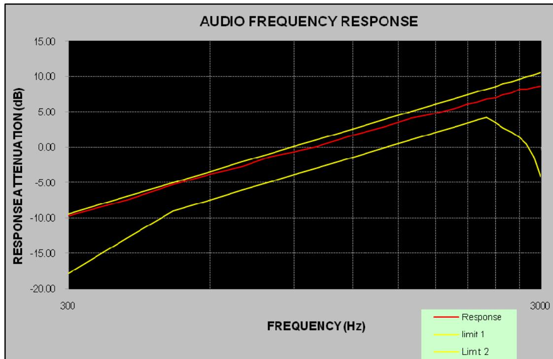
Carrier Frequency: 450.0125 MHz, Channel Separation=12.5 kHz
