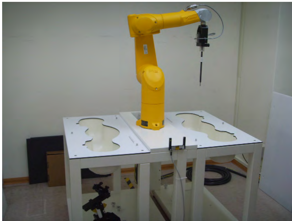
Fig.1 Photograph of the SAR measurement system
