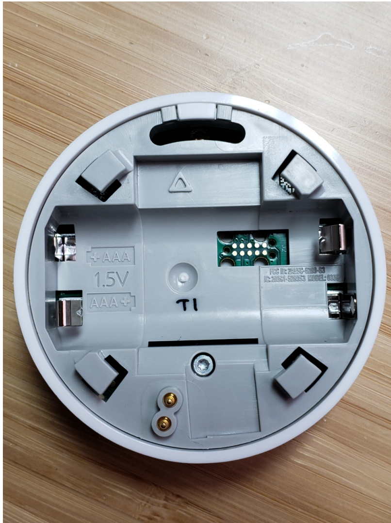
Figure 4, back, battery cover / mount removed, note FCC / IC IDs molded in.
