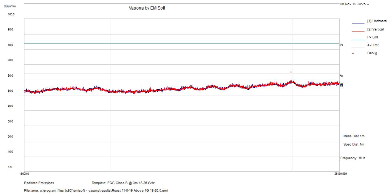
*Worst Case Colocation: TRTN 50 kbps 2-GFSK, 25 kHz deviation, IEEE 802.15.4g MR-FSK PHY mode 915 MHz and LTE Band 4 mid channel 1732MHz*
