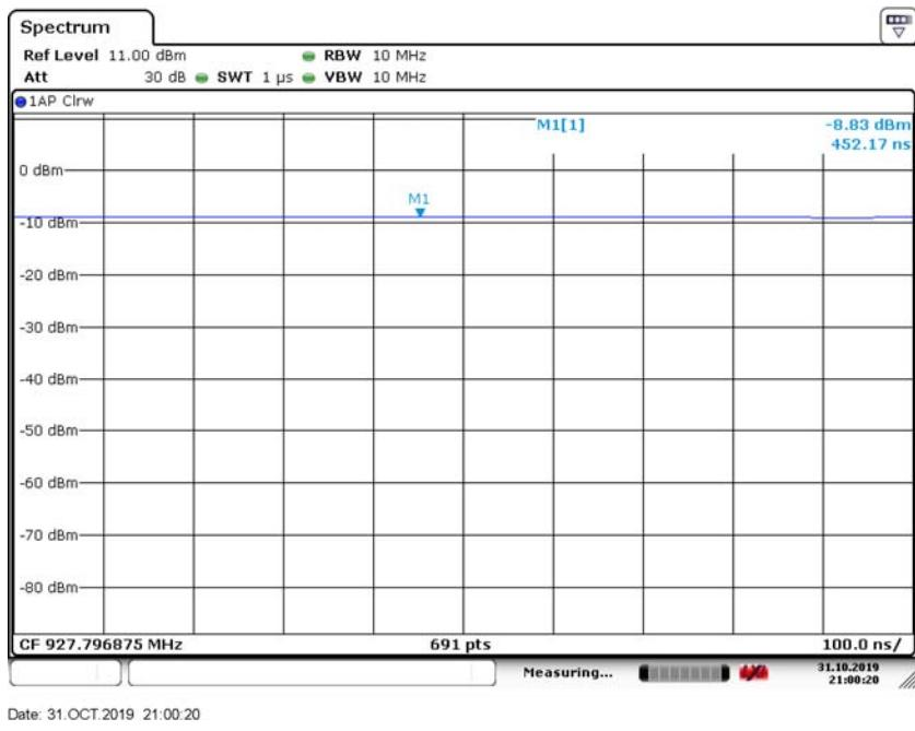
**5 kbps, SimpleLink Long Range (20 kchip/s, 2-GFSK, conv. FEC r=1/2 K=7 DSSS SF=2, Tx dev:5 kHz, RX BW: 49 kHz)**
