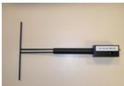
Figure 1 – Satimo COMOSAR Validation Dipole
