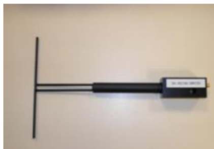
Figure 1 – Satimo COMOSAR Validation Dipole
