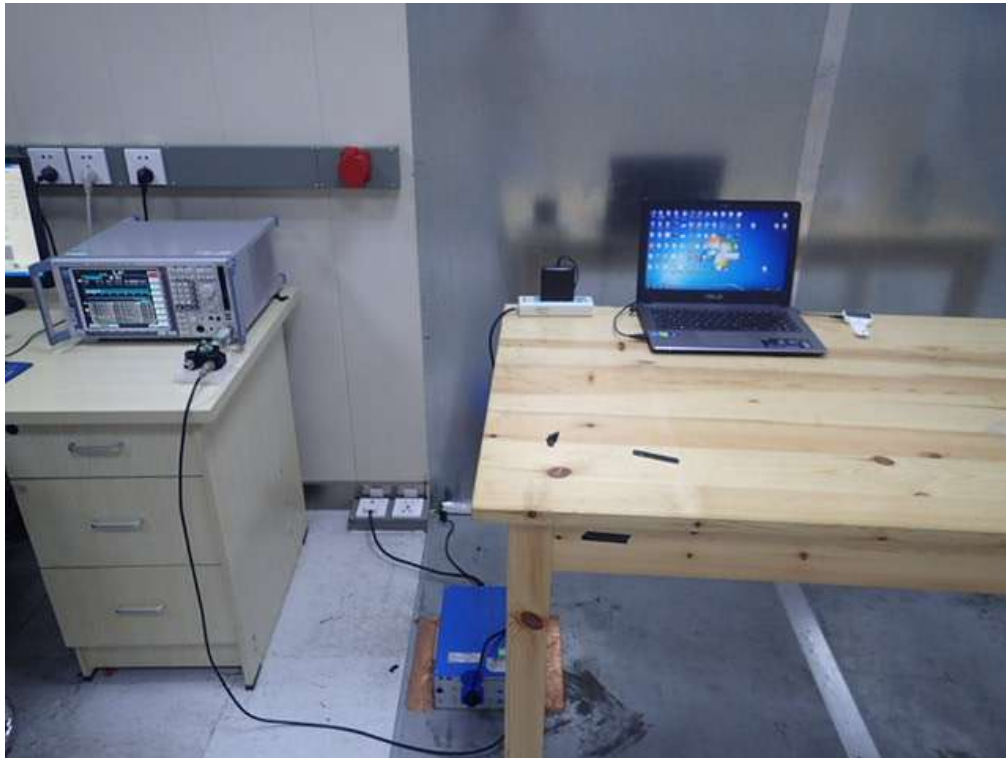
FCC RADIATED EMISSION TEST SETUP
