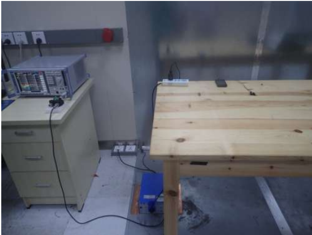
FCC RADIATED EMISSION TEST SETUP
