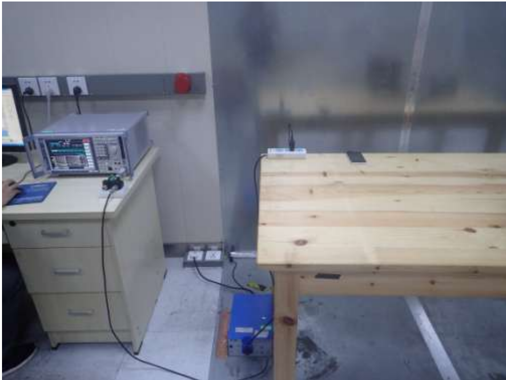
FCC RADIATED EMISSION TEST SETUP
