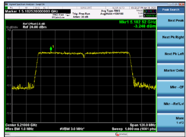
(802.11ac80) PSD plot on channel 42
