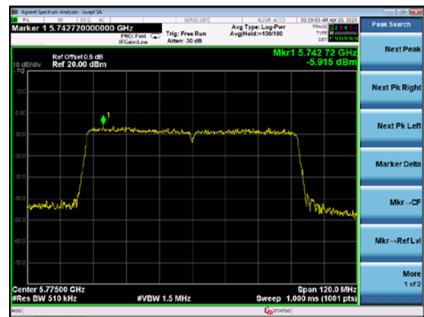
(802.11ac80) PSD plot on channel 155
