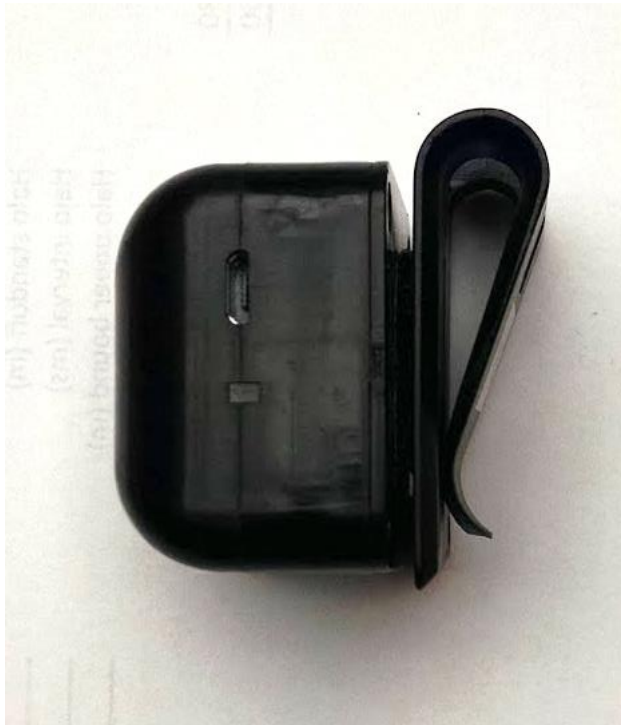
Transmitter with Clip (Note: Clip is plastic, affixed via velcro)
