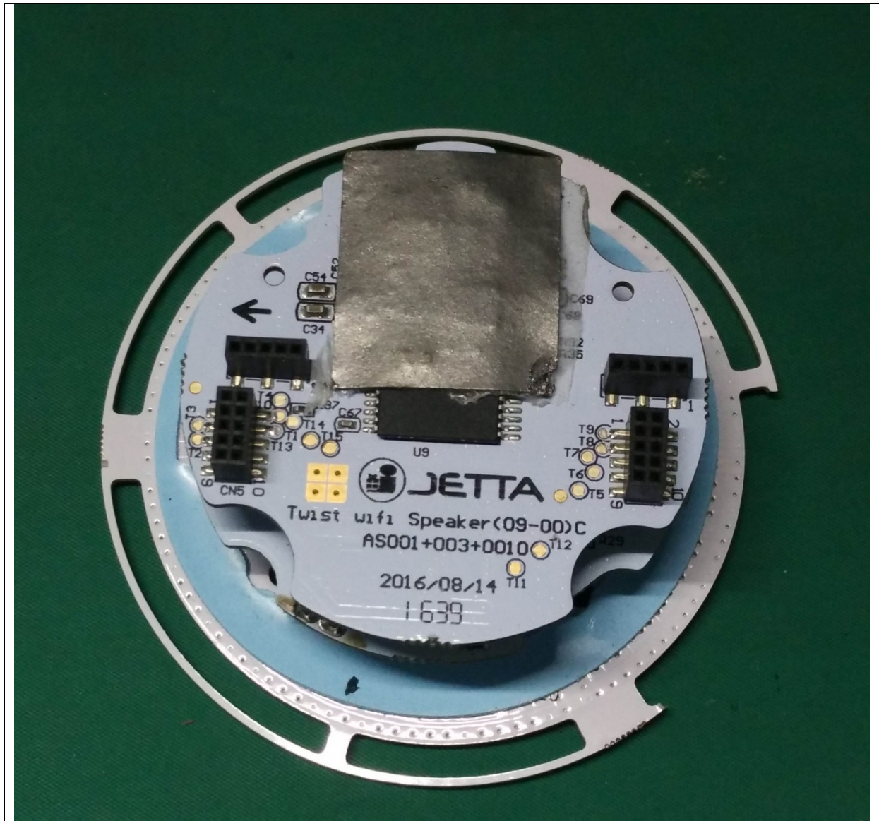
WiFi Board Bottom with RF Absorber
